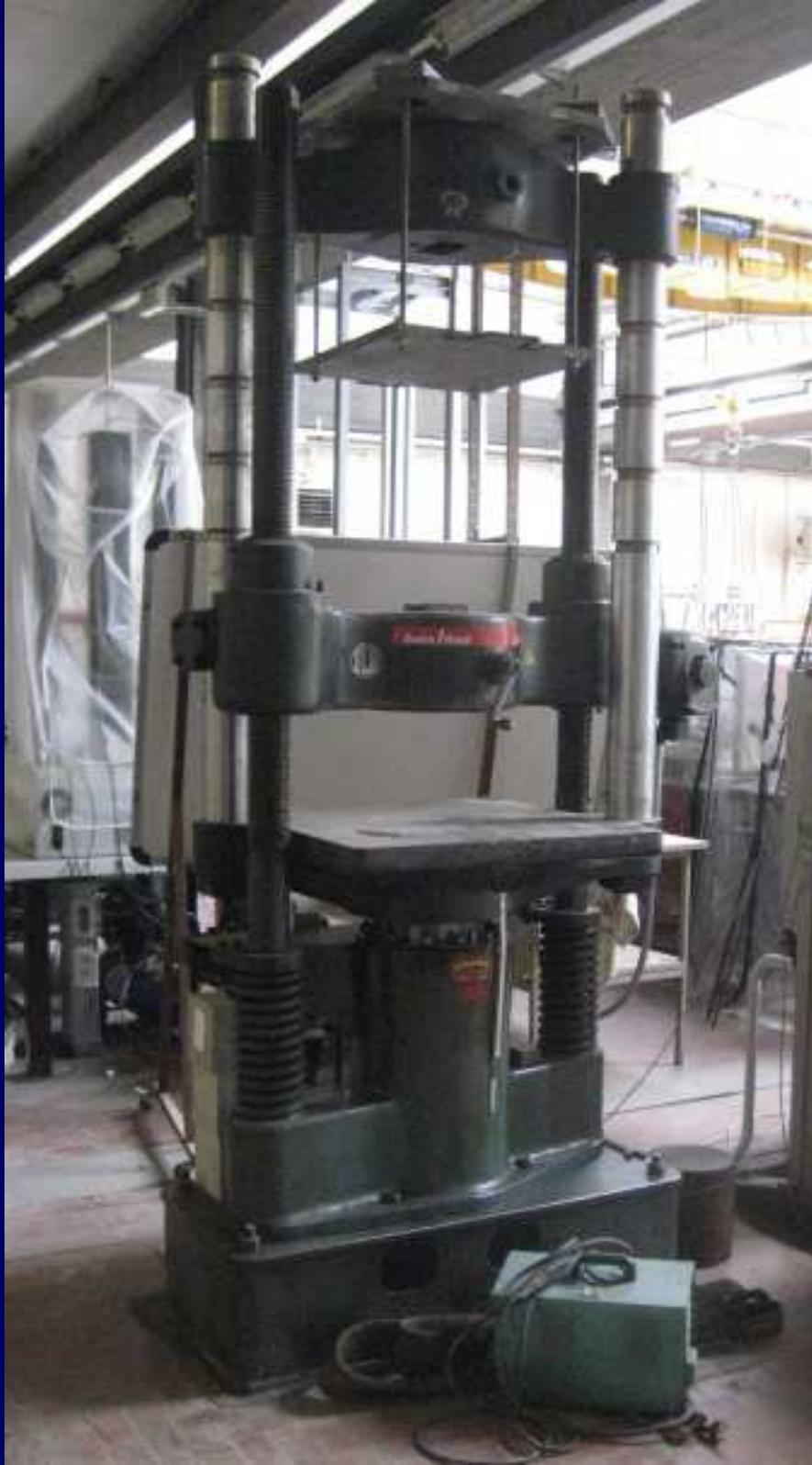
The same testing machine was used on all the test specimens: a standard servo-hydraulic press Baldwin with a maximum capacity of 500 kN, equipped with control electronics.
