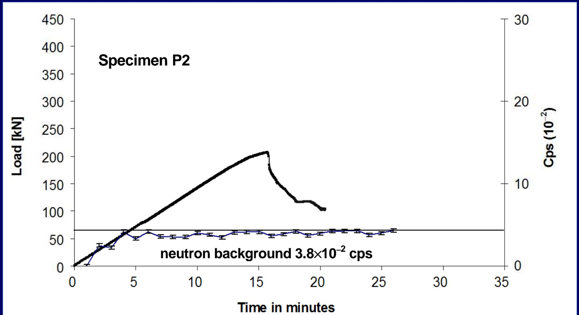
Load vs. time and cps curve for P2 test specimen in Carrara marble.
