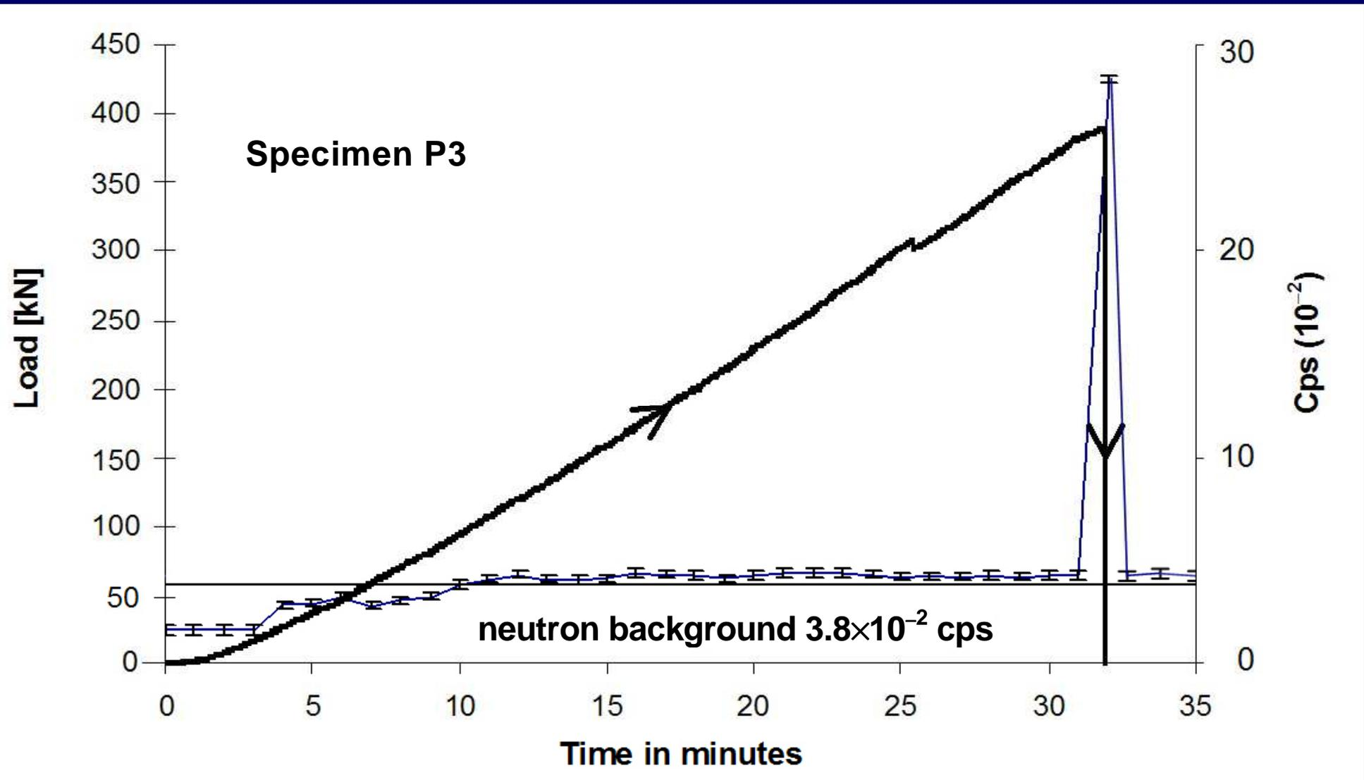
Load vs. time and cps curve for P3 test specimen in Luserna granite.
