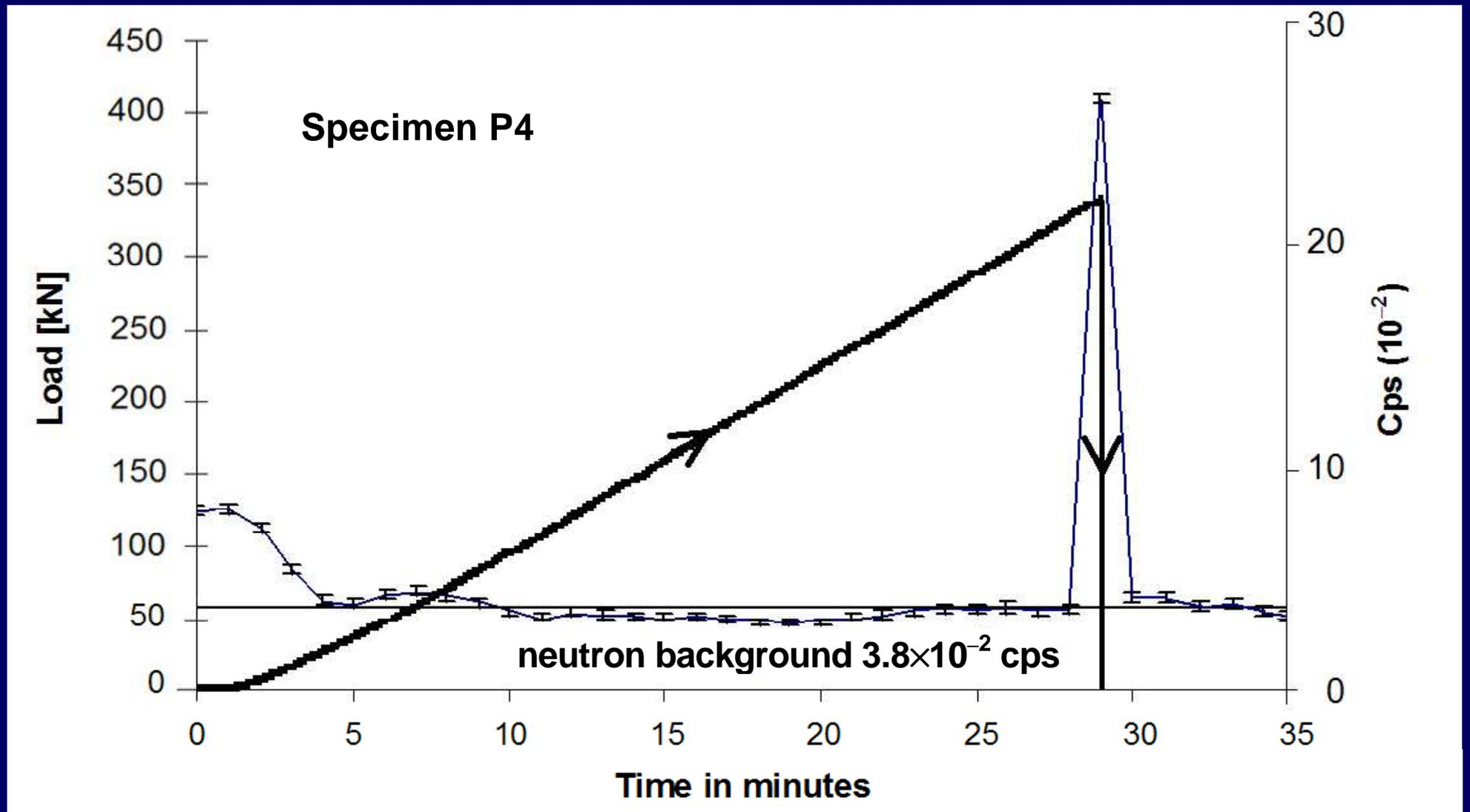
Load vs. time and cps curve for P4 test specimen in Luserna granite.
