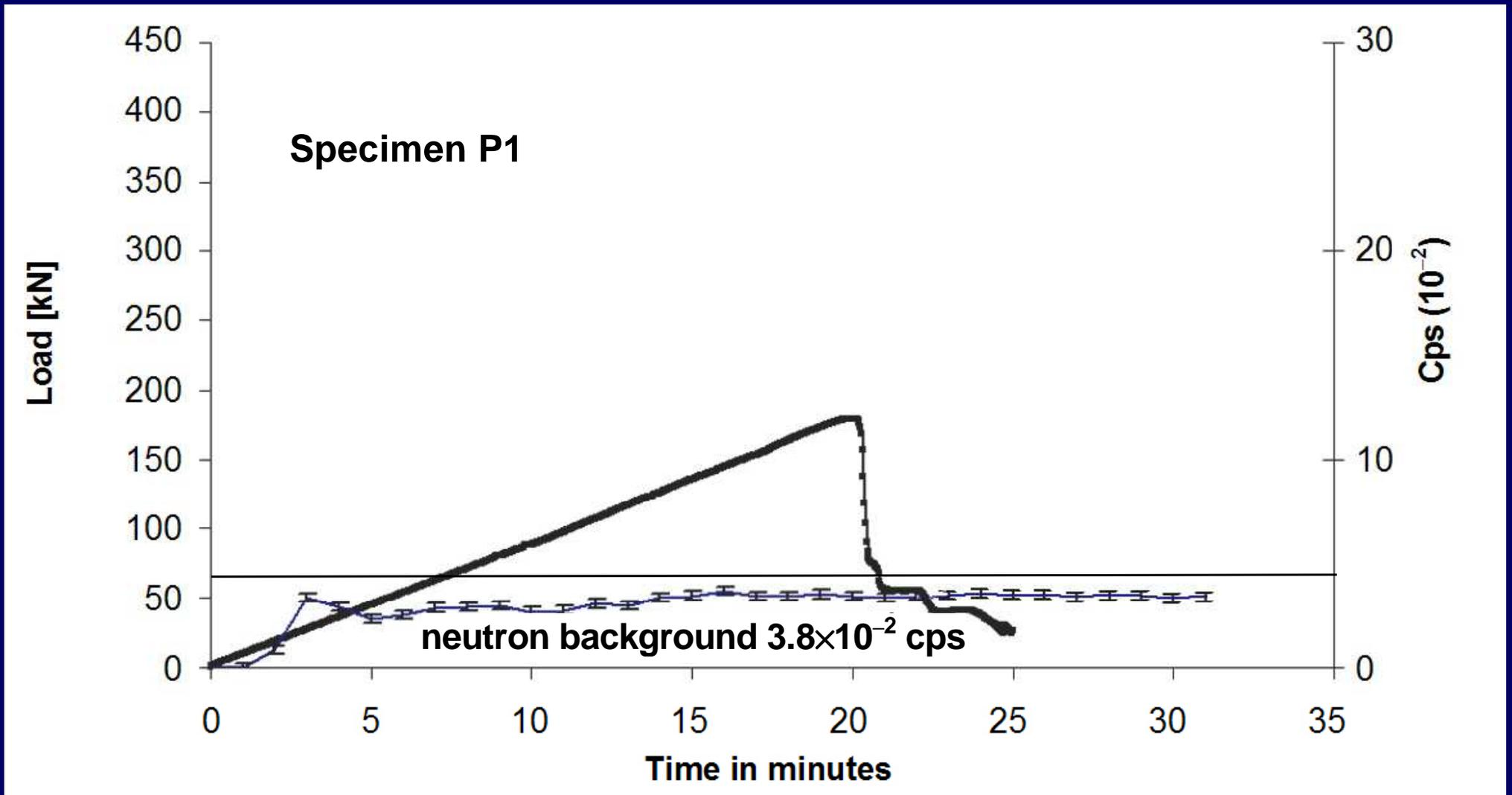
Load vs. time and cps curve for P1 test specimen in Carrara marble.
